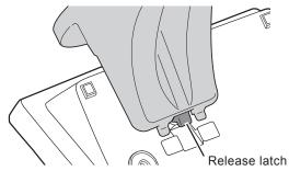
Note: Mounting the phone directly on the wall
